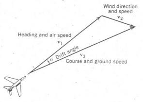
The length of vector  $v_1$  represents the plane's air speed and the direction of vector  $v_1$  shows the heading. The length of vector  $v_2$  shows the speed of the wind and the direction of vector  $v_2$  shows the direction of the wind. The length of vector  $v_3$  shows the ground speed and the direction of vector  $v_3$  shows the course.
